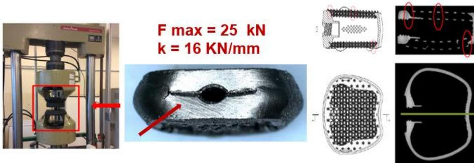
Fig. 3. Exemplary research results: A) mechanical properties and microscopic analysis until rupture of the implants, B) cross-section through implants taking into account critical areas using the technical computed tomography system CT
