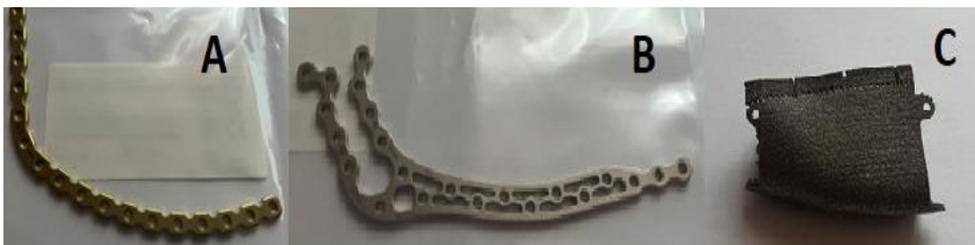
Fig. 1. Types of plates used: A-standard plate (Modus M-4566), B-openwork plate (Modus M2-4603), C-personalized implant
