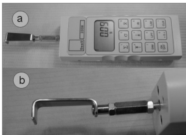
Fig. 5. Electronic force gauge TesT model 320: a – general view of the gauge with a contact tip enabling hooking up the incisors, b – side profile of the tip
