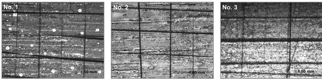
Fig. 6. Macroscopic view of AISI 316L specimens coated with sol-gel layers No. 1 to 3 after adherence testing
