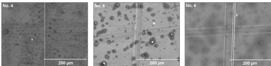
Fig. 9. Surface of AISI 316L specimens coated with sol-gel layers No. 4 to 6 after adherence testing. No sign of cracking proves good adherence to the base. SEM
