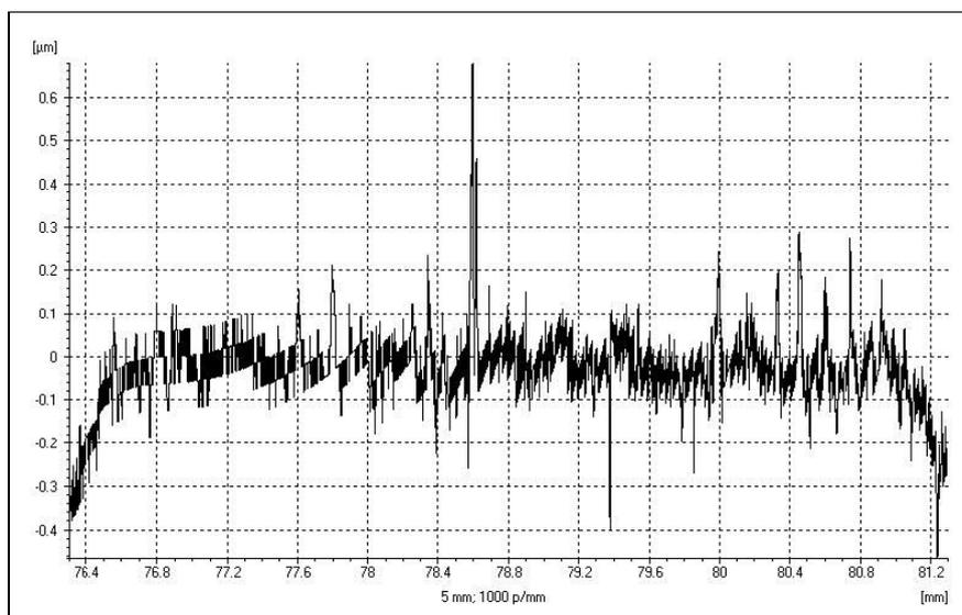
Fig. 11. Surface profilogram of a steel specimen
