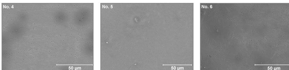
Fig. 5. Surface of AISI 316L steel specimens coated with sol-gel layers No. 4 to 6 after deformation. Slip lines and bands created during tension are visible under the coatings. SEM
