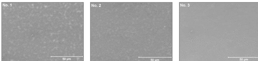
Fig. 2. Surface of AISI 316L steel specimens coated with sol-gel layers No. 1 to 3 before deformation. The defects in the form of numerous uniformly distributed pores are visible. SEM
