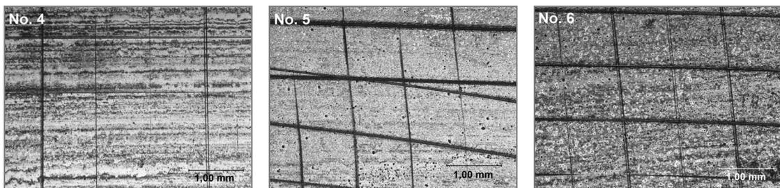
Fig. 8. Macroscopic view of AISI 316L specimens coated with sol-gel layers No. 4 to 6 after adherence testing
