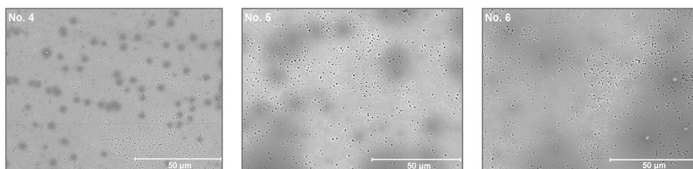
Fig. 4. Surface of AISI 316L steel specimens coated with sol-gel layers No. 4 to 6 before deformation. The defects in the form of numerous uniformly distributed pores are visible. SEM
