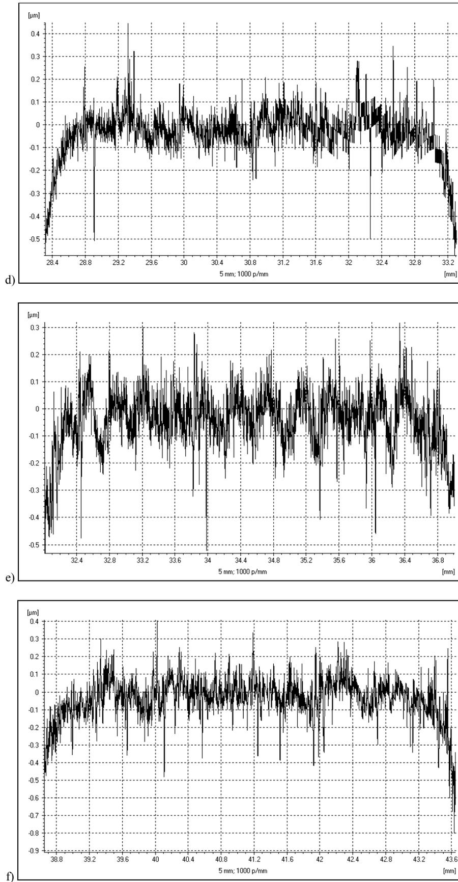
Fig. 10. Two-dimensional surface profilograms of steel specimens coated with silica sol-gel layers
