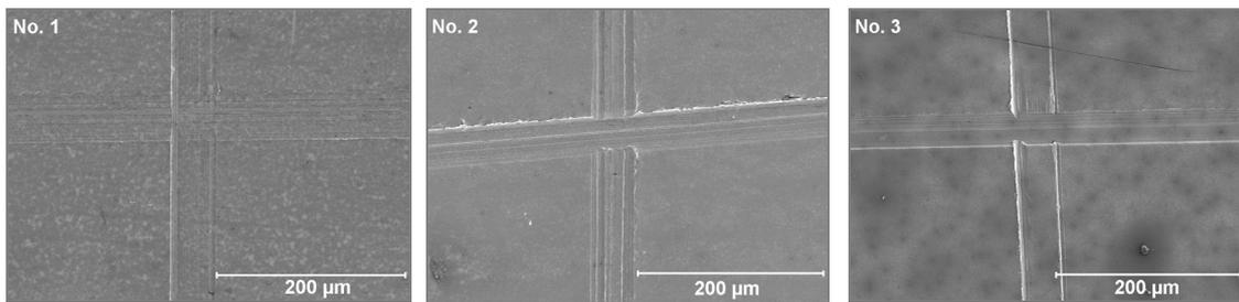
Fig. 7. Surface of AISI 316L specimens coated with sol-gel layers No. 1 to 3 after adherence testing. No sign of cracking proves good adherence to the base. SEM
