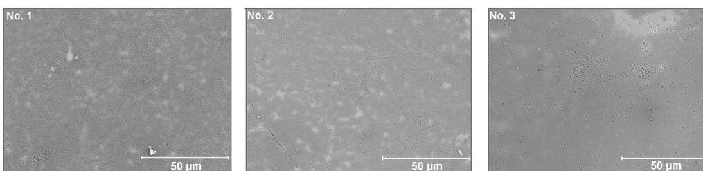
Fig. 3. Surface of AISI 316L steel specimens coated with sol-gel layers No. 1 to 3 after deformation. The slip lines and bands created during tension are visible under the coatings. SEM
