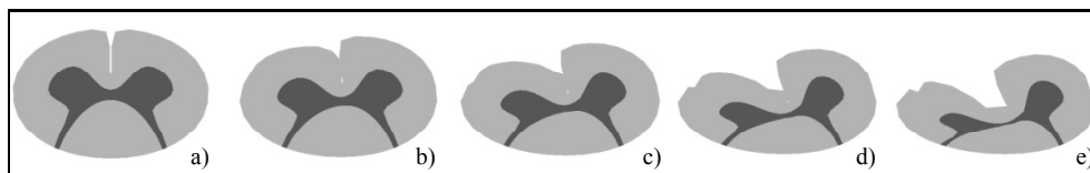
Fig. 7. Finite Element Model of the cervical spinal cord. Deformation of spinal cord cross-section in the region of load application: a) original shape of model cross-section, b) deformation caused by 25% of maximal loading, c) deformation caused by 50% of maximal loading, d) deformation caused by 75% of maximal loading, e) deformation caused by maximal loading
