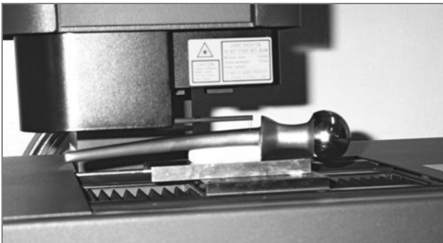
Fig. 1. Surface testing of Weller endoprosthesis stem
