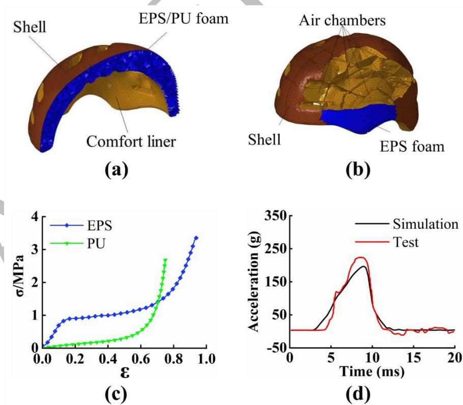
Figure 2. The FE modes of the EPS/PU (a) and airbag (b) helmet, the stress-strain curves of EPS and PU material (c) and the validation result of the EPS helmet model (d).
