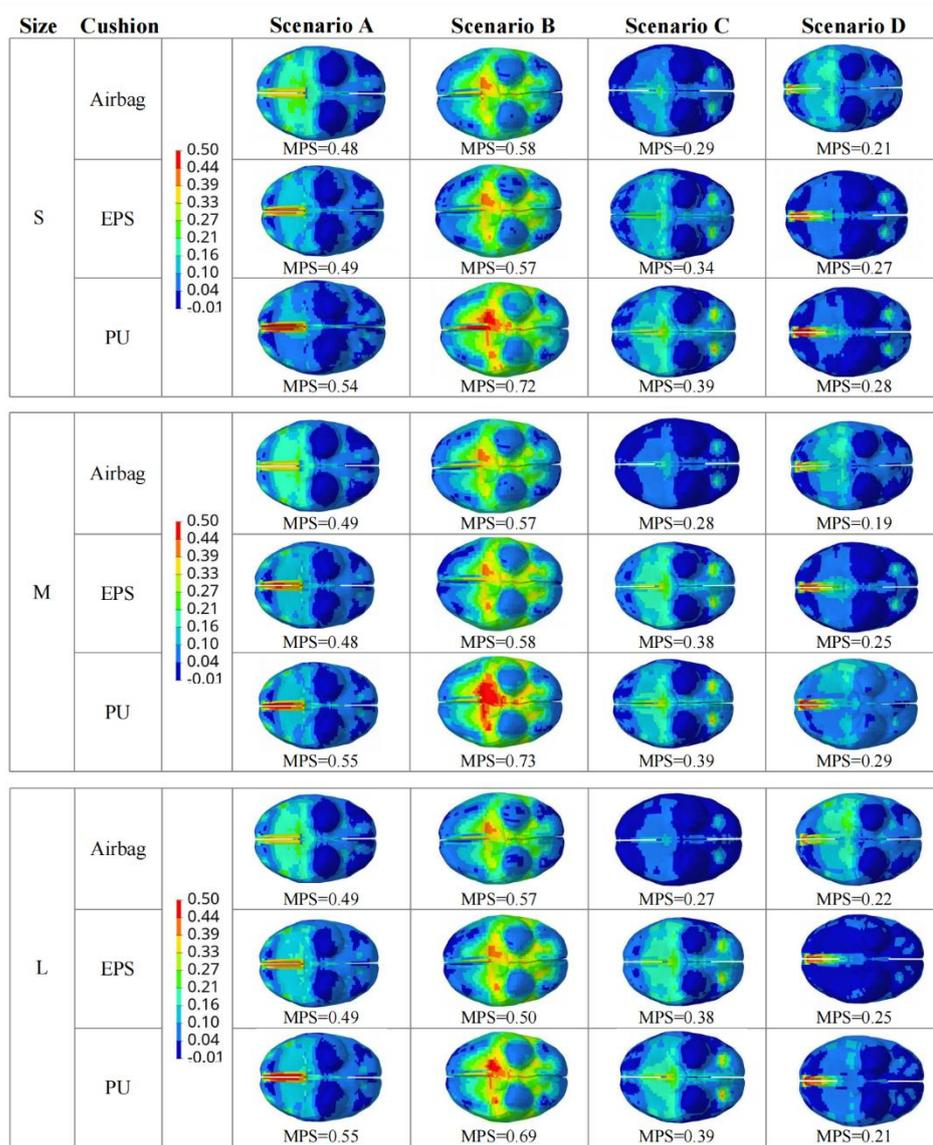
Figure 6. The predicted brain strain distribution and MPS values of all impact simulations.
