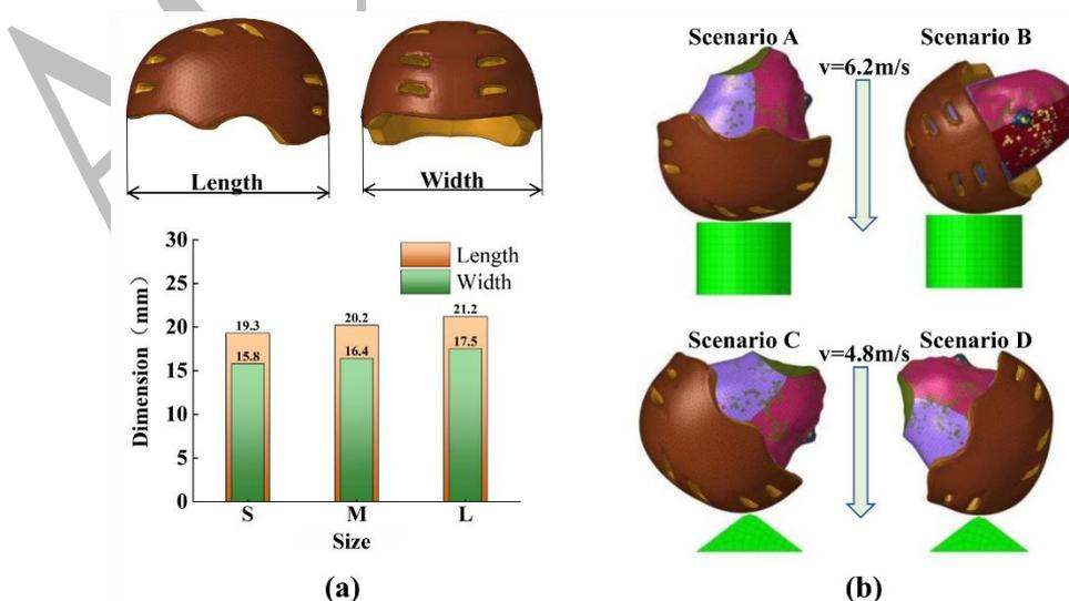
Figure 3. The dimensions of the helmets in different sizes (a) and the impact scenarios (b).
