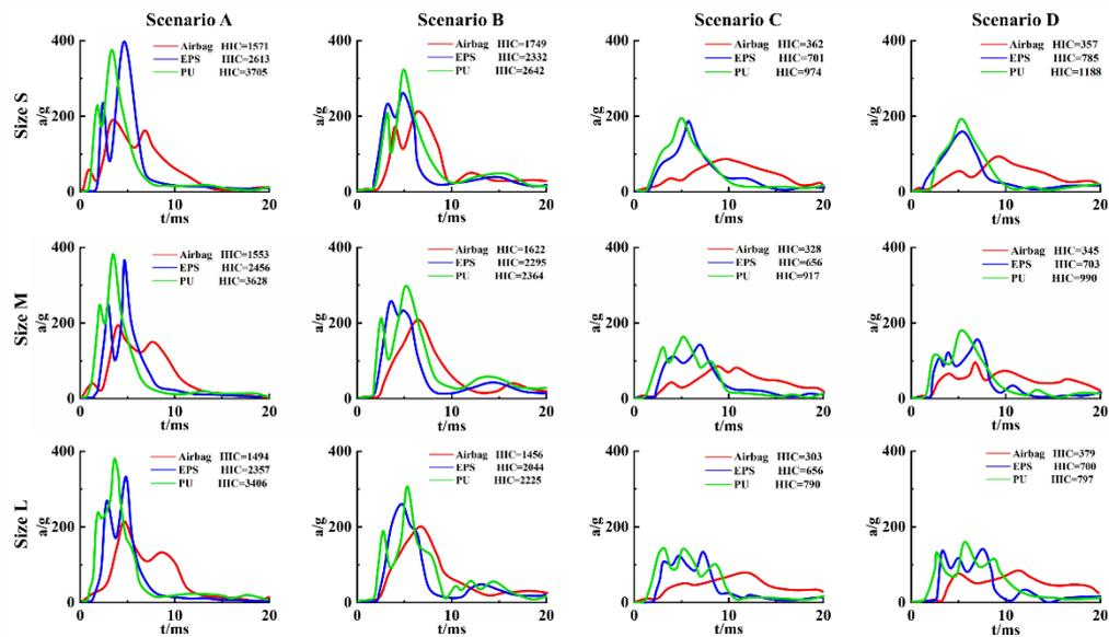
Figure 4. The predicted head linear acceleration curves and HIC values of all impact simulations.
