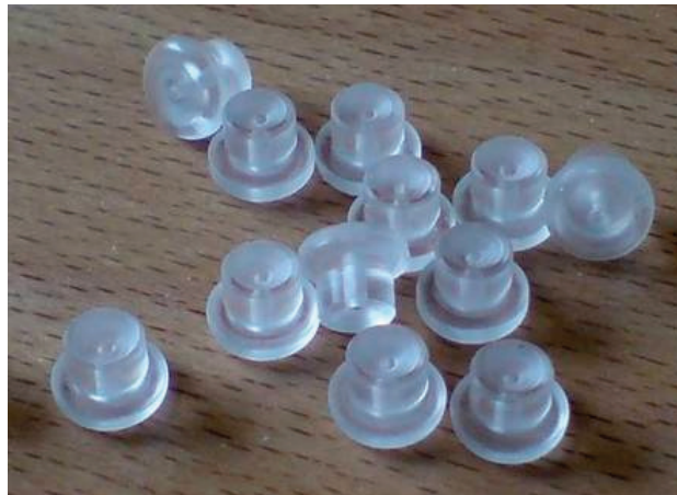
Fig. 2. Poly (2-hydroxyethylmethacrylate) scaffolds – upper parts of replacements
