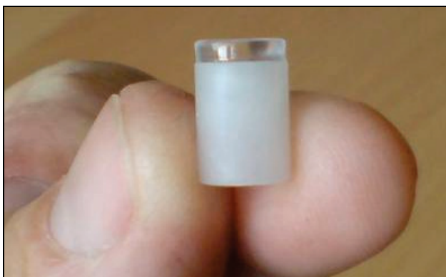
Fig. 1. Bi-component replacement of the subchondral bone (in the distal part, nontransparent material) and the articular cartilage scaffold (partly, in the proximal part, transparent hydrogel)
