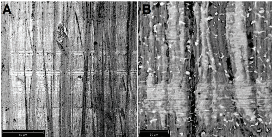
Fig. 12. Surface of the Ti6Al7Nb alloy rod: A – visible uneven distribution of pressures in the friction area, B – smoothing of the surface caused by flattening the tops of the uneven structure; friction in the presence of acidic sodium lactate
