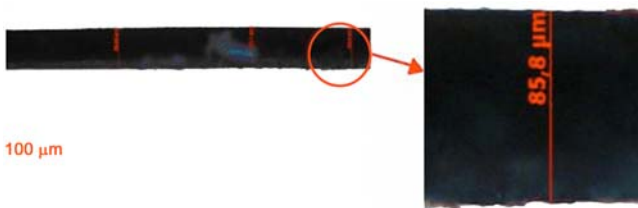
Fig. 1. Way of determining hair's diameter from optical microscope image
