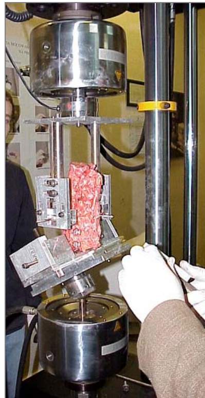
Fig. 1. Testing spine fixed on spine tester
