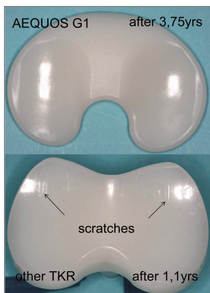
Fig. 8. Explanted tibia-inlays. Above: AEQUOS-inlay explanted after 3.75 years. Scratches could not be seen. Below: inlay from a one of the most common conventional TKR explanted after 1.1 years in which significant stress marks were seen
