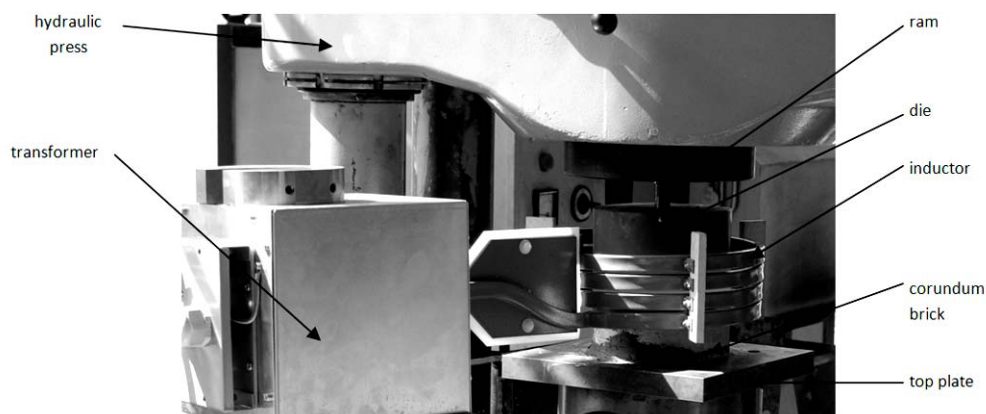
Fig. 3. Device for argon-shielded hot pressing of titanium and titanium alloy powders
