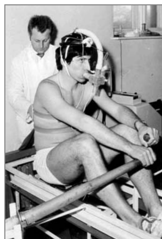
Fig. 8. Universal Rowing Ergometer UEW-1 used for biomechanical and physiological tests of the rowers
