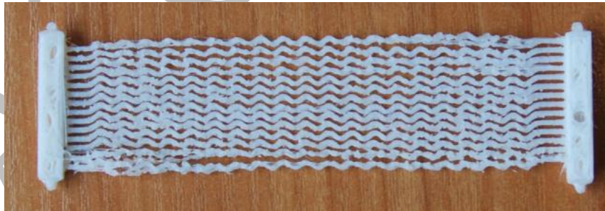
Figure 6. Fiber arrangement in the inner layer of the material sample with fixing elements.
