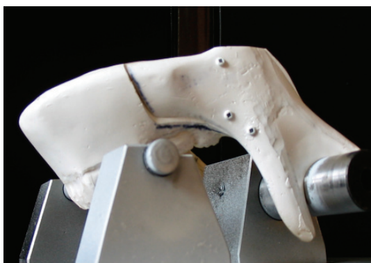
Fig. 4. Scheme of the mandible model loading
