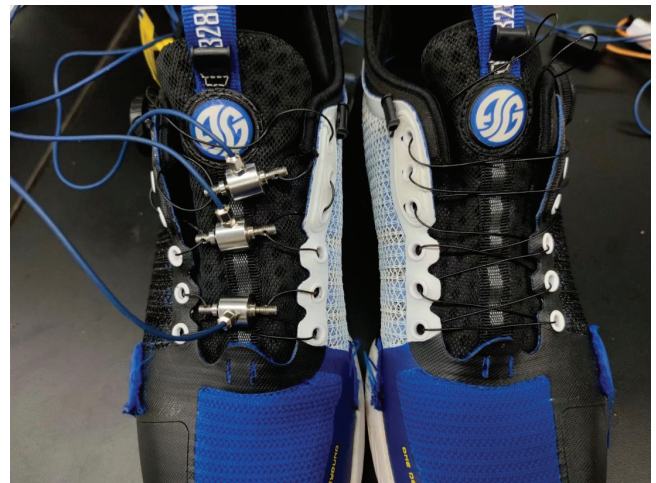
Fig. 2. Three micro force transducers placed in this study
